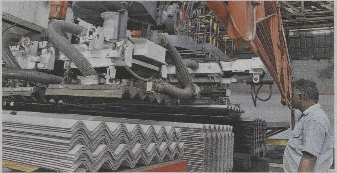
HIL's automatised production line for asbestos roofing sheets at Sanathnagar in Hyderabad. PV SIVAKUMAR
